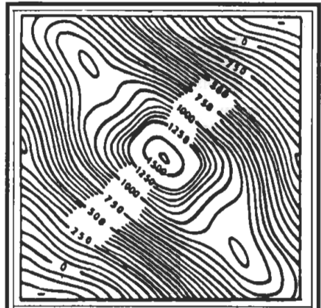
FIG. (8.b). Autocorrelogram of the thorium map of G. Idid El Gedan area, North Eastern Desert, Egypt.
